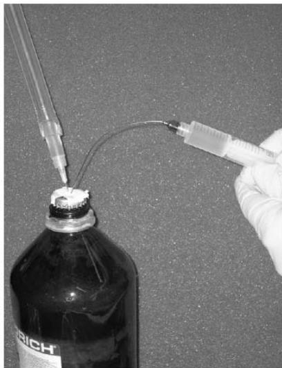
*Fig 3. Inert gas bubbles and excess liquid are forced back into reagent bottle*
